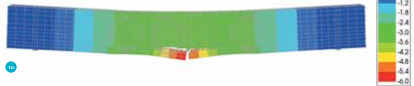
15684_basismodel load-step 105, load-factor 54.000, LC2_load displacements TD+Z min: -6.2 mm max: 0.9 mm
