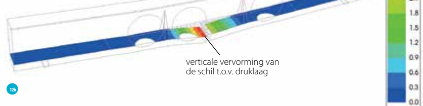
15684_basismodel load-step 105, load-factor 54.000, LC2_load interface relative displacements DUNz min: -0.0 mm max: 3.0 mm
