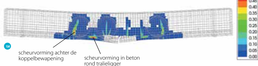
15684_basismodel load-step 105, load-factor 54.000, LC2_load crack-widths Ecw1 min: -0.00 mm max: 0.91 mm
